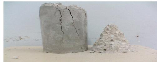
**Figura 5.** (concreto com borracha e EPS)
